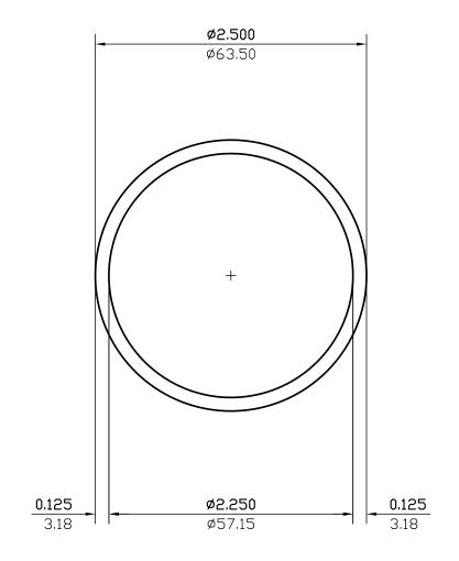
0.125 (3.18) WALL THICKNESS EXCEPT AS SHOWN DATE REV DESCRIPTION BY 03/10/23 2 REMOVED ALLOY NDZAL 08/05/99 REDRAWN PAUL 601.720 мм.2 EST.AREA 0.933 IN.<sup>2</sup> EST.AREA 1.638 1.101 EST.WT. LBS/FT. EST.WT. KG/M. 14.923 379.033 EST.PER. EST.PER. MM. 7.854 199.5 OUT PER. OUT PER. MM. 2.500 63.500 C.C.D. C.C.D. M/F FINISH ALLOY
